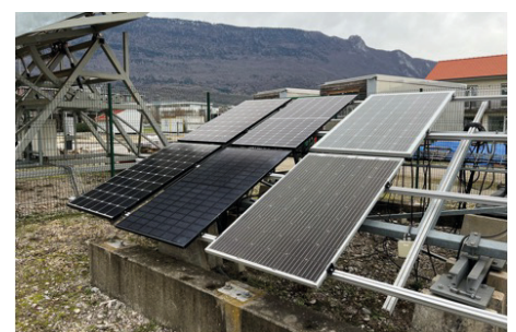
Fig. 2: PID outdoor tests on 6 PV modules.
